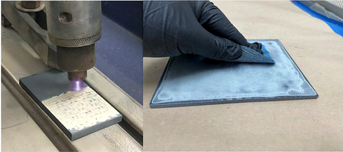
Figure 11: Plasma coating removal being performed on smaller cutout piece for parameter DoE (left) and hand sanding being performed (right)
