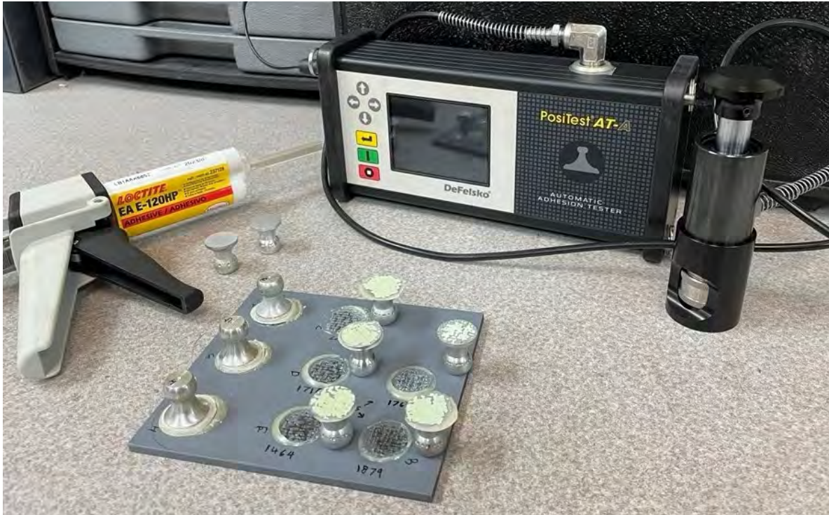
Figure 17: Defelsko Positest AT-A used for pull-off strength adhesion testing
