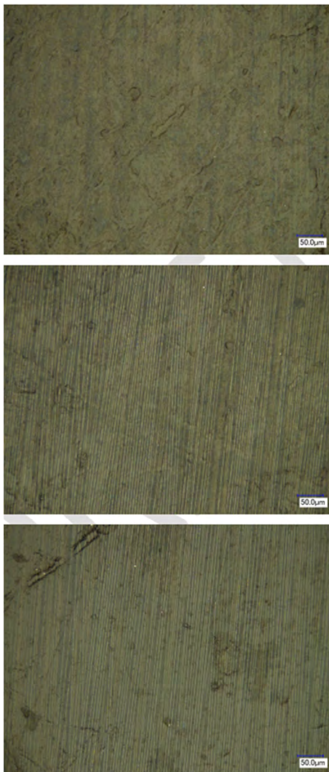
Figure A2: Bare Carbon Fiber Control Specimen 500x
