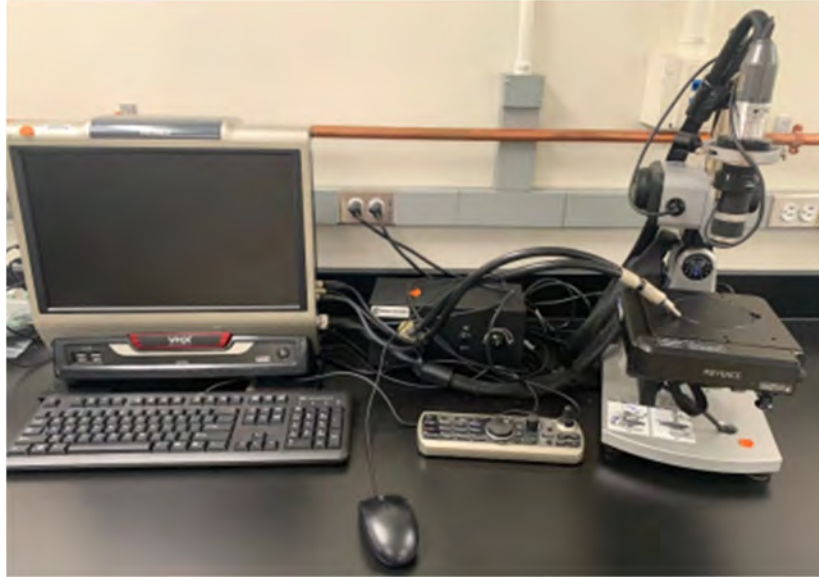
Figure 12: Keyence VHX Digital Multi Scan Microscope used to take photomicrographs and generate 3D surface profiles.
