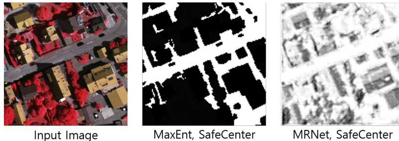
Figure 9: Results of SafeCenter training for MAXENT IRL [164] and MRNET. With high cost regions marked in black, we can see that unlike MAXENT where transition between obstacles and driveable space is sharp, MRNET has gradual transition between the two regions, favoring center of the road then edge of roads.
