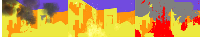
Figure 24: An example of provided labels for fire cases. Dark gray: smoke (soft label), light yellow: fire (soft label), gray: smoke, red: fire, yellow: furniture, orange: wall, purple: ceiling. The soft label represents a highly detailed transparency-preserving segmentation of flame and smoke.
