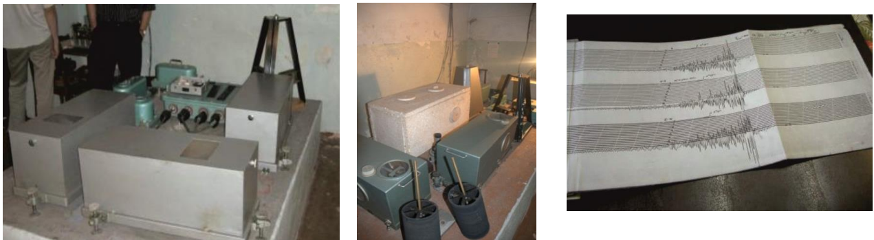
Figure 4. Kirnos SKM-3 seismograph with a magnification V=20000 , installed at the Frunze (FRU) seismic station in Bishkek, and an example of a recorded seismogram.
