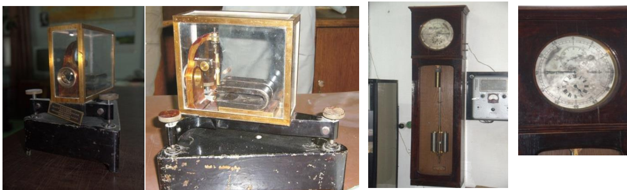
Figure 2. Seismograph with direct optical registration, designed by P. Nikiforov. Frunze station (FRU) of the Institute of Seismology of National Academy of Sciences of the Kyrgyz Republic (1927-1950, NS, EW components).
