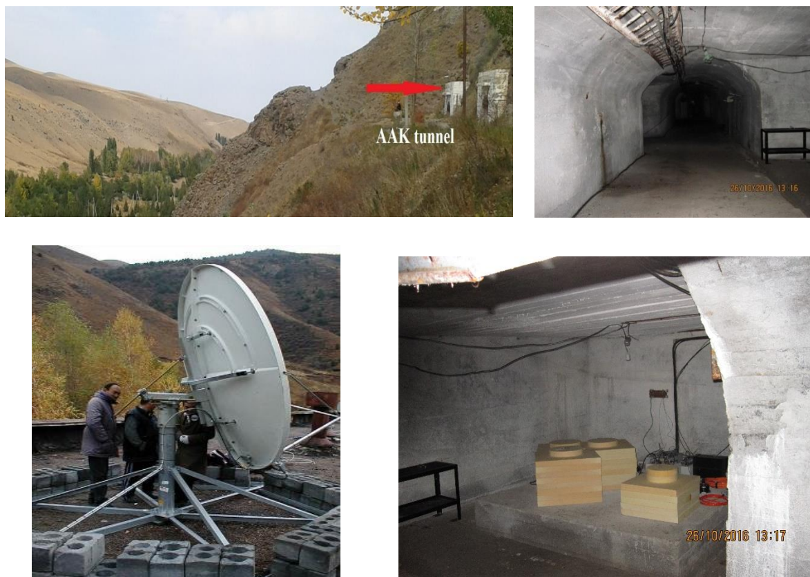
Figure 5. Photos of the GSN station AAK showing tunnel location, tunnel, telemetry antenna, and sensor pier.
