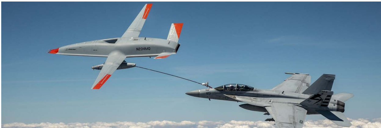
Figure 6: MQ-25 Autonomous tanker refueling an F-18 Superhornet. Boeing, 2022
