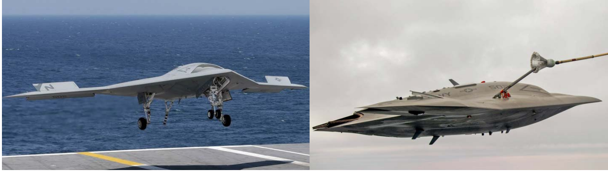
Figure 7: X-47B landing on an aircraft carrier and refueling in flight. Northrop Grumman, 2023
