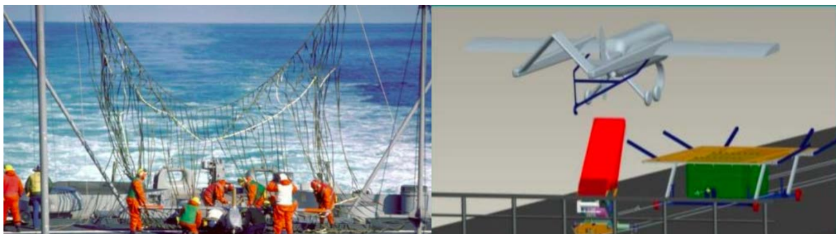
Figure 15: UAS net recovery and arrestor wire concepts, Boeing, 2022.
