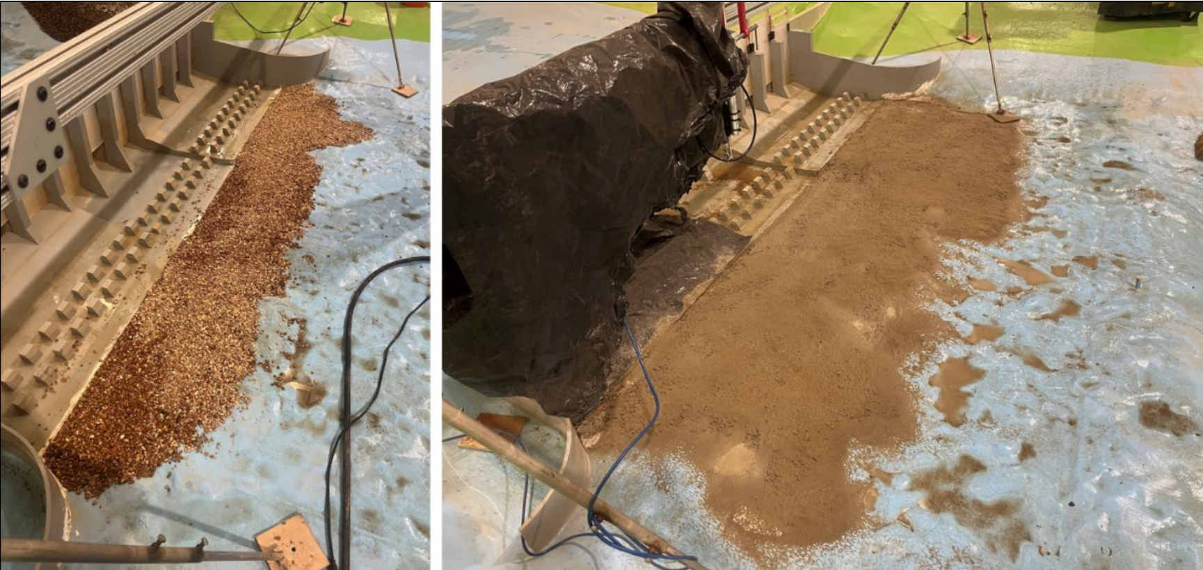
Figure 7. Model modifications (pre-cement dusting on the left and post-cement dusting on the right ).
