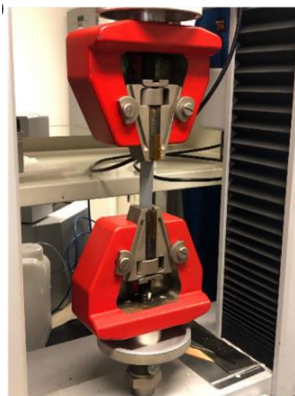
Figure 16. Test configuration for measuring the elastic properties of the different coating samples.
