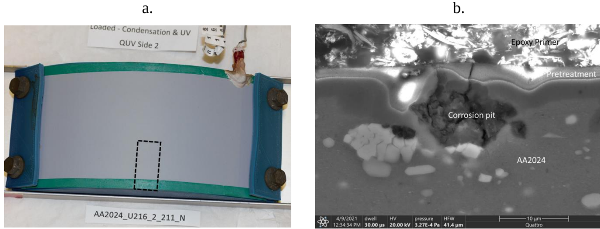
Figure 29. a. Test panel following 2184 hours of UV and condensation exposure with sampling region highlighted. b. SEM image of a corrosion pit found below a crack in the surface pretreatment on a 2% strained coating system.
