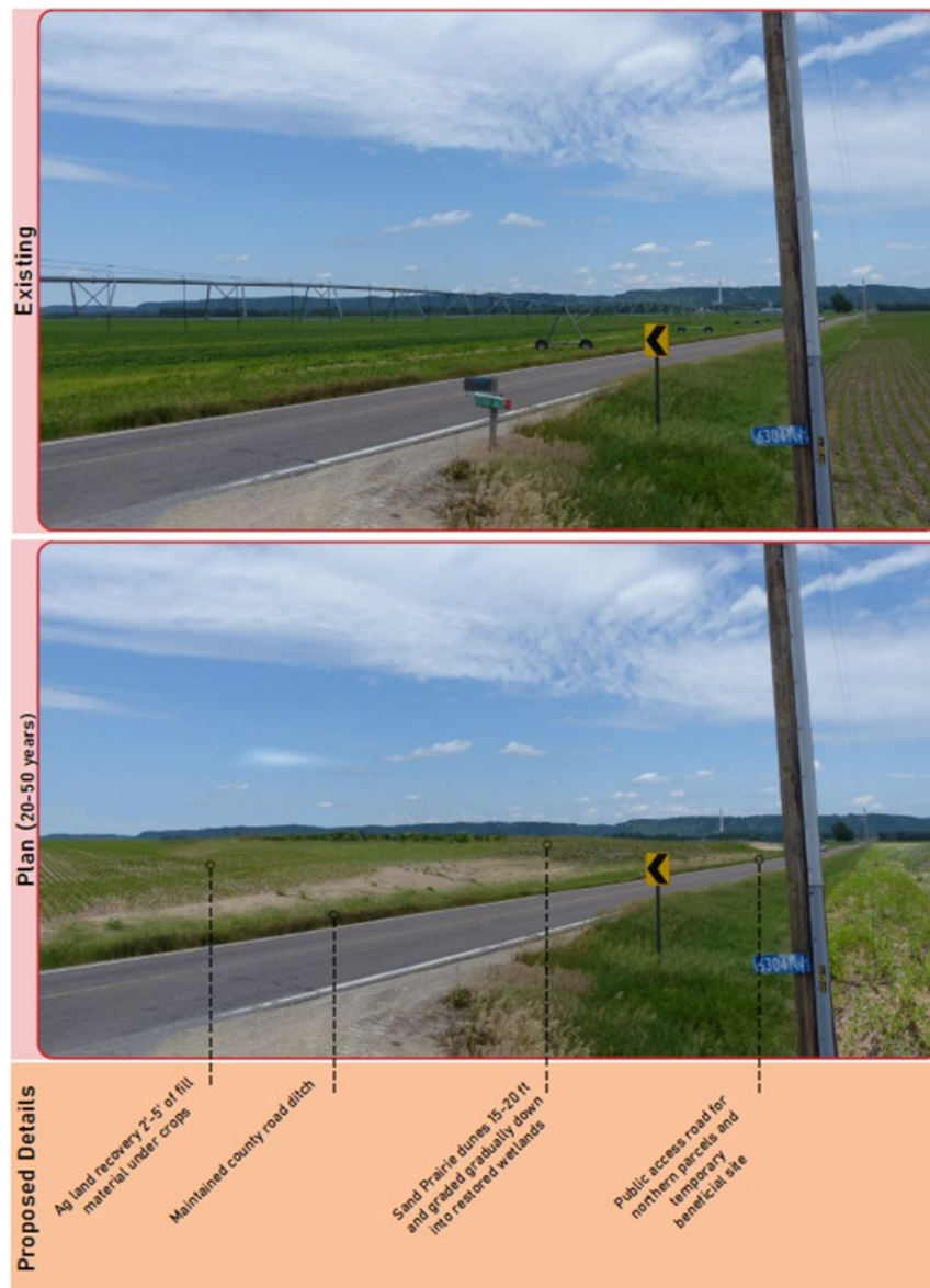
Figure 7. Rolling Prairie dredged sediment placement for the cropland recovery area shown in Figure 3. Top photo shows the existing land use; the bottom photo is a rendering of the desired end state.
