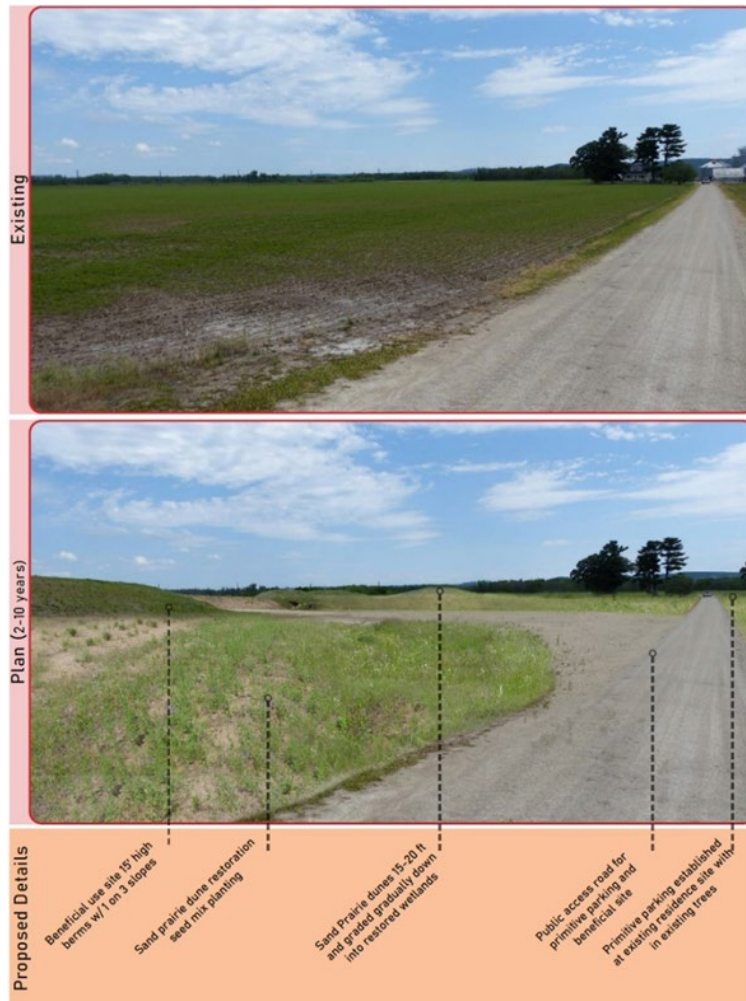
Figure 6. Rolling Prairie location where the public will be able to access dry dredged sediment placed here for public or commercial uses. Top photo shows the existing land use; the bottom photo is a rendering of the desired end state.
