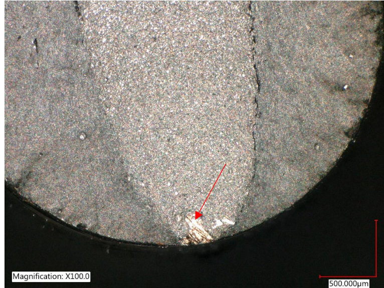
Figure 3 Fracture surface of the tensile specimen with the lowest ductility (sample 17)
