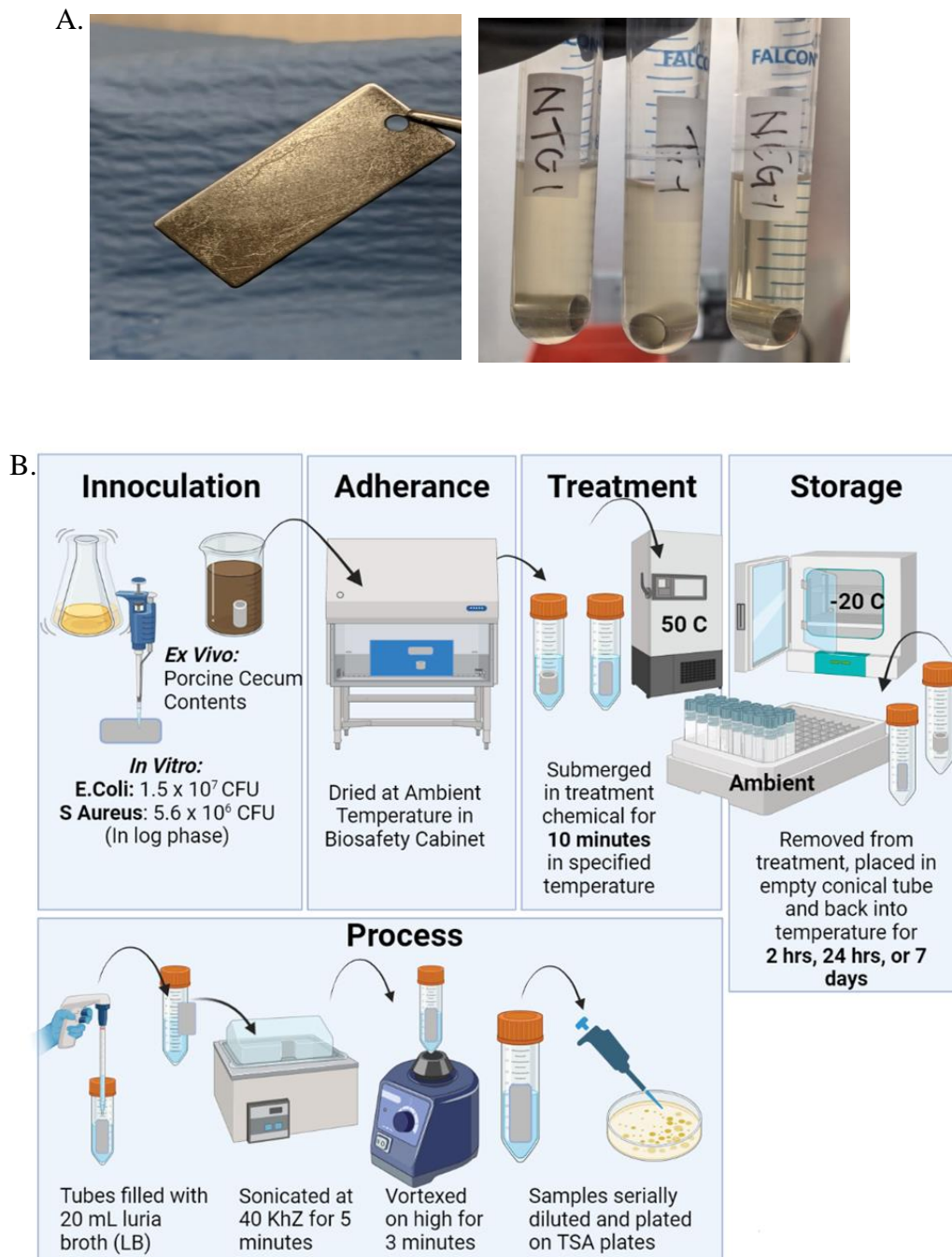
Figure 1. A. Stainless steel test coupons (left) and stainless steel peni-cylinders submerged in bacteria containing broths (right) used in the experiment. B. Schematic of experimental design created using BioRender.com.
