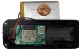
Fig 1. ESP32 processor with 512 KB of onboard memory
