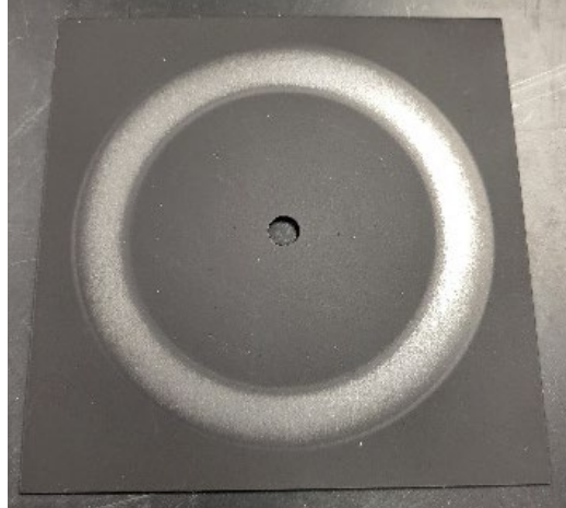
Fig. 12 Cerakote C-192 following 4000 cycles of Taber abrasion
