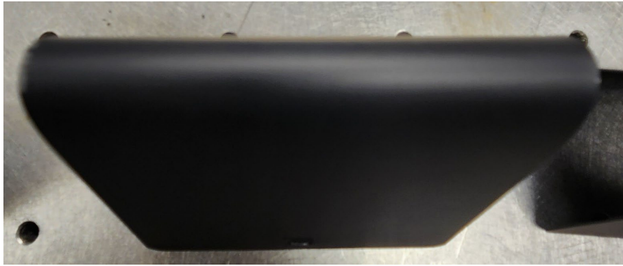
Fig. 5 Cerakote C7600 following mandrel bend
