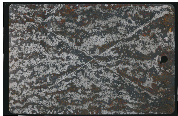
Fig. 18 DuraCoat DuraHeat 2.0 at 800 °F after ASTM B117 exposure
