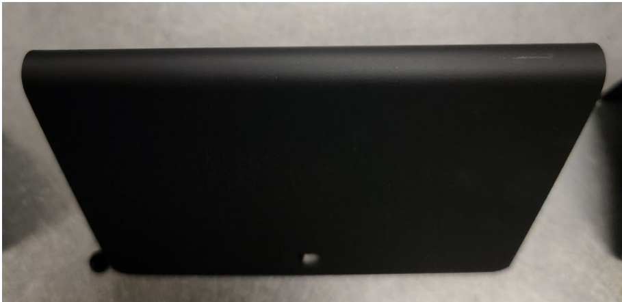
Fig. 7 DuraCoat DuraHeat 2.0 following mandrel bend
