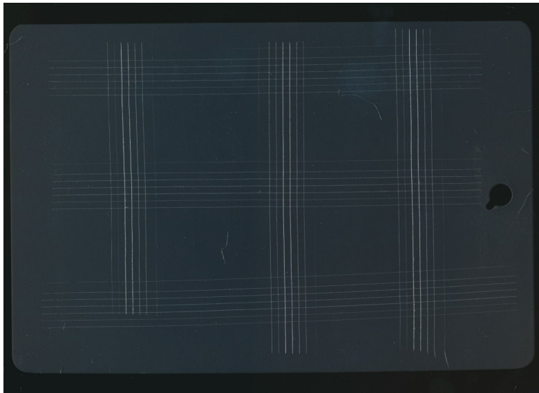
Fig. 8 Cerakote C-192 cross-hatch adhesion results
