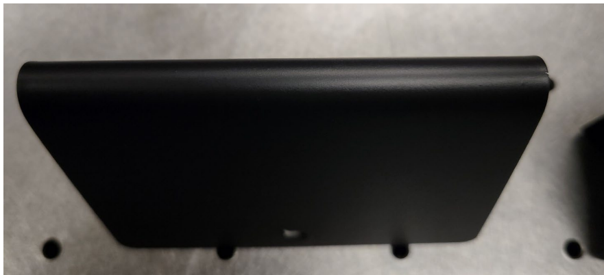
Fig. 4 Cerakote C-192 following mandrel bend
