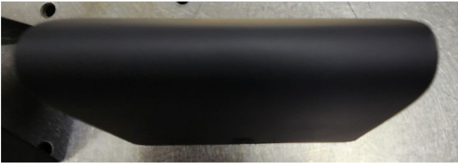
Fig. 6 Cerakote V-169 following mandrel bend
