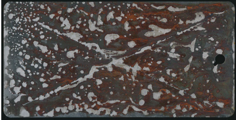
Fig. 16 Cerakote C7600 at 800 °F after ASTM B117 exposure
