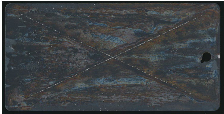
Fig. 17 Cerakote V-169 at 800 °F after ASTM B117 exposure
