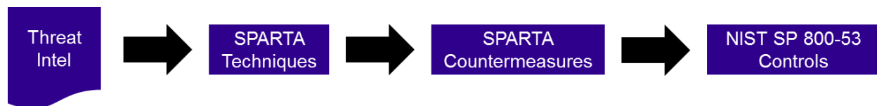
Figure 5 - Threat Linkage to Controls
