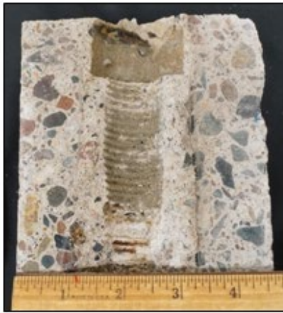
(a) Heavy deterioration around the second nut
