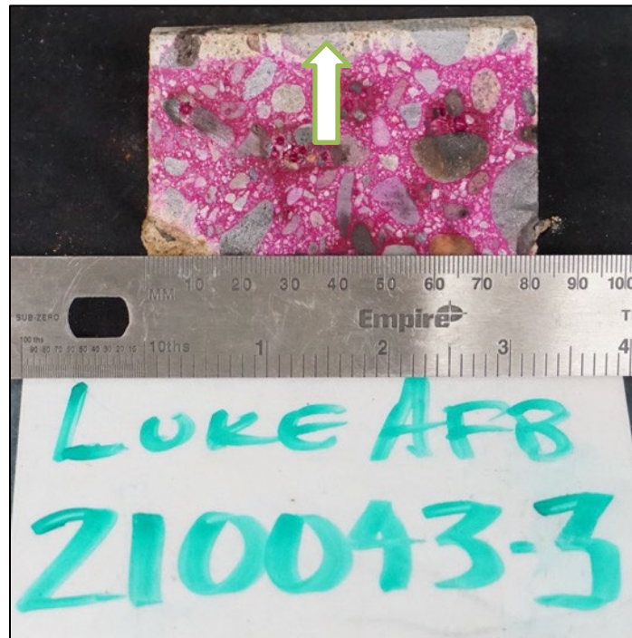
Figure 34. Phenolphthalein applied to sample 210043-3.
