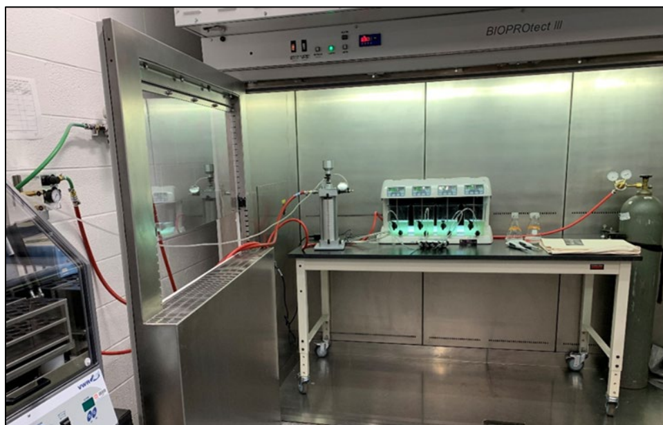
Figure 8. Physical experiment set-up for bench-scale CO 2 -enhanced DAF jar testing.
