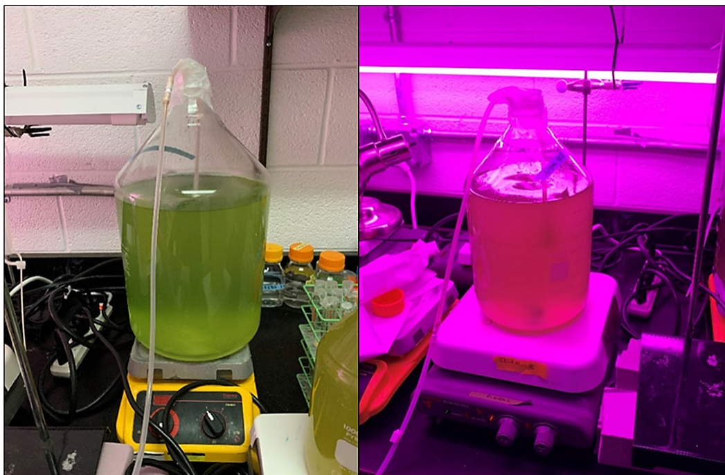
Figure 4. Algae cultivation setup with growth lights off ( left ) and on ( right ).
