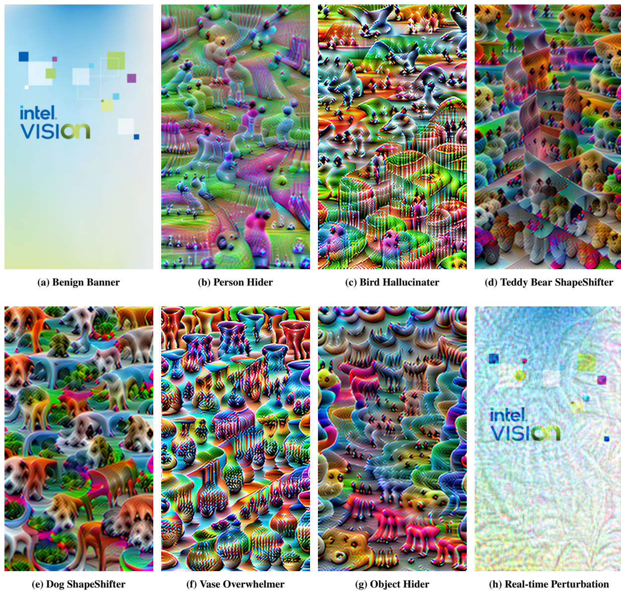
Figure 3.17: The patches we generated using MART. Each patch had a different adversary goal as described in their respective captions. See Figure 6.3 for example detections from our demo. The real-time perturbation (h) mimics the setup of the current GARD evaluations. As such, it requires less perturbation budget than the other patches and thus looks more like the benign banner (a).
