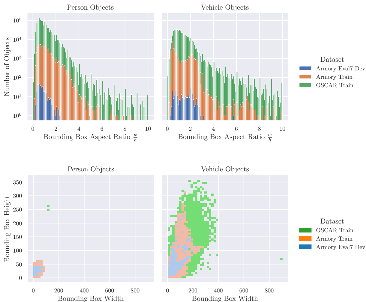
Figure 3.26: Annotation statistics for our collected dataset (OSCAR Train) versus the provided training dataset (Armory Train) versus the provided development/test dataset (Armory Eval7 Dev) by annotation category (person/pedestrian and vehicle). While the provided training dataset covers person/pedestrian detections well, our training dataset covers many more vehicle sizes (as measured by bounding box width and height) and orientations (as measured by bounding box aspect ratio).
