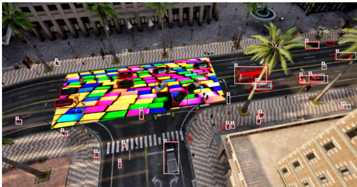
Figure 3.32: Adversarial gemstone patch sampled using end-to-end optimization. The resulting patch is completely natural and un-perturbed by high frequency noise, while still ensuring the overlaying vehicles are missed by the object detector.
