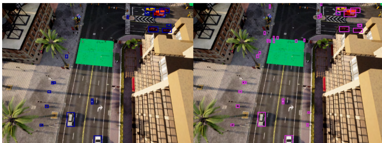
Figure 3.1: An example image with 18 original bounding box annotations (marked in blue) is missing person annotations that are visibly walking on the sidewalk and the patch (left). Augmenting these annotations to include all objects reveals all 33 annotations (marked in magenta, right).
