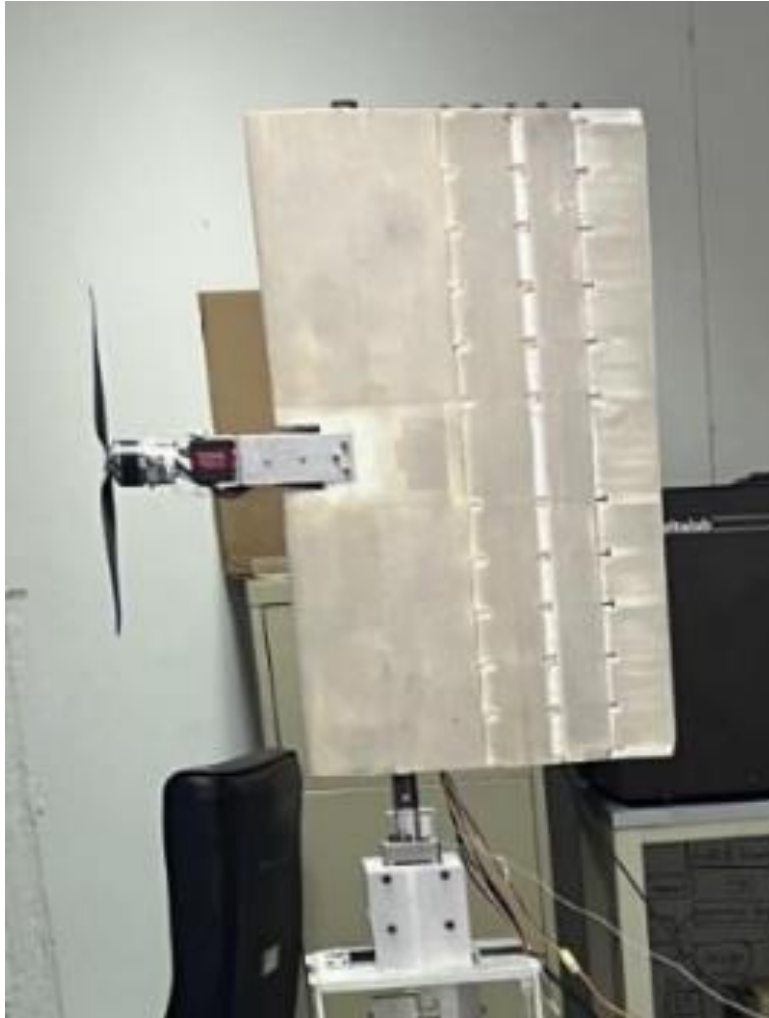
Figure 17: Wing Part (Wing, Control surface, motor mounting, transducer, and motor-propeller)
