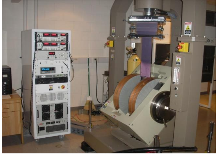
Fig. 22: 2.2 Tesla vector vibrating sample magnetometer used for measurements of field and temperature (100 K to 350 K) dependence of magnetization.
