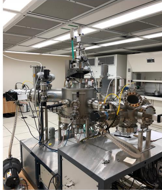
Fig. 13: Multitarget sputtering system with load-lock used for deposition of \text{FeCo} , \beta\text{-W} and \text{Bi}_2\text{Te}_3 films (base pressure \approx 8 \times 10^{-9} \text{ mbar} ).
