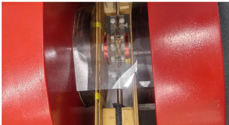
Fig. 2(b): Top view of the waveguide placed between Helmholtz coils and the pole pieces of a 1.5 tesla electromagnet.
