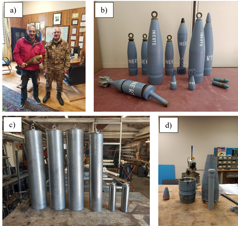
Figure 6. a) Professor Maurizio Brocchini and Colonel Luca Corrieri at the “Stabilimento Militare Ripristini e Recupero del Munizionamento”; b) inert ammunitions painted in "Steel Blue"; c) steel cylinders built by a local blacksmith; d) 155mm projectile cut to place the instrumentation (grey cylinder in foreground) into it.
