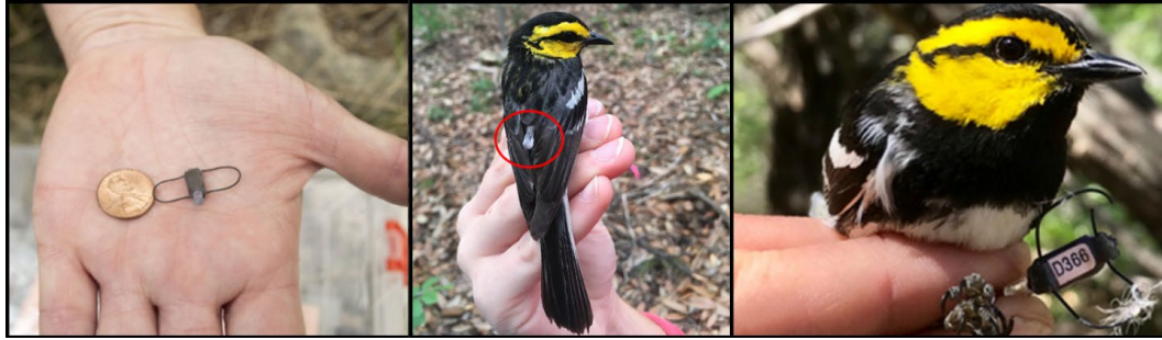
Figure 3. Left: Geolocator with a 5-mm light stalk and leg-loop harness (0.41 g). Center: Geolocator attached to male golden-cheeked warbler ( Setophaga chrysoparia ). Right: Geolocator retrieved from a male golden-cheeked warbler the year after it was attached.
