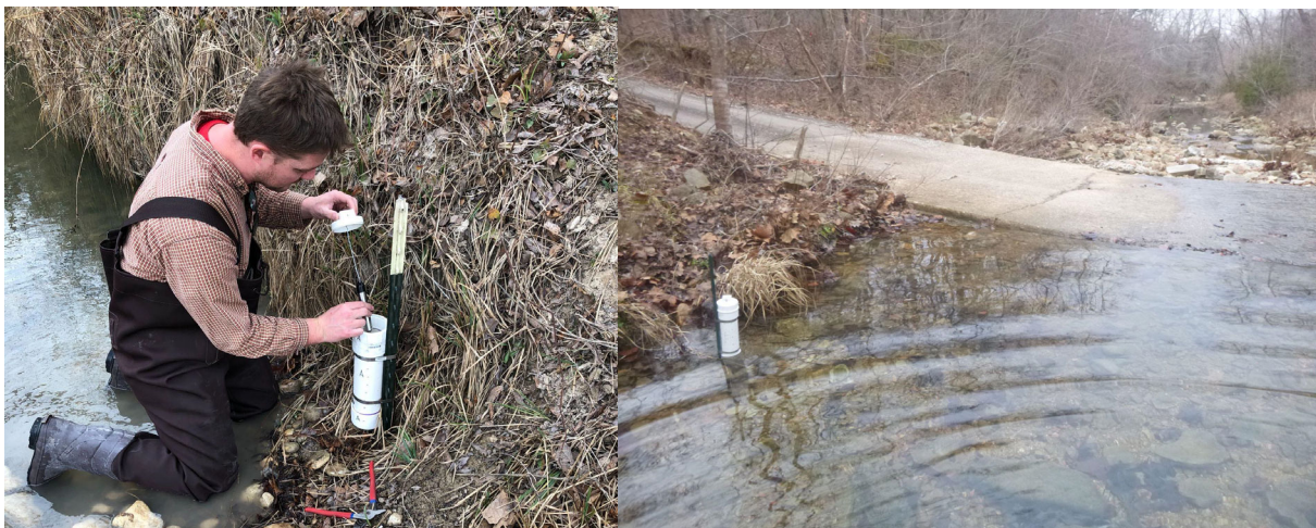
Figure 5.1: HOBO water depth data loggers deployed on Table Rock Creek at Fort Hood, TX and on Turnbull Hollow at FLW, MO.
