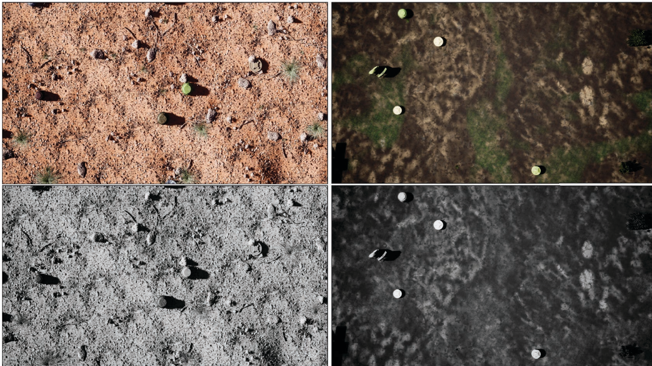
Figure 4: Example 2022 GEQ data – top is RGB, bottom is corresponding grayscale – produced procedurally 32 in support of this article. Compared to our old simulated imagery (see Figure 3), this new data has more realistic objects, textures, illumination, shadows, and the overall quality is more photo-realistic.
