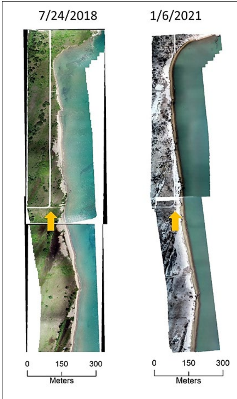
Figure 4. Unmanned aerial vehicle (UAV) imagery collected from the beginning and end of the study used for ground truth shoreline data. Note the strong erosion over the time interval and loss of the road (gold arrow).
