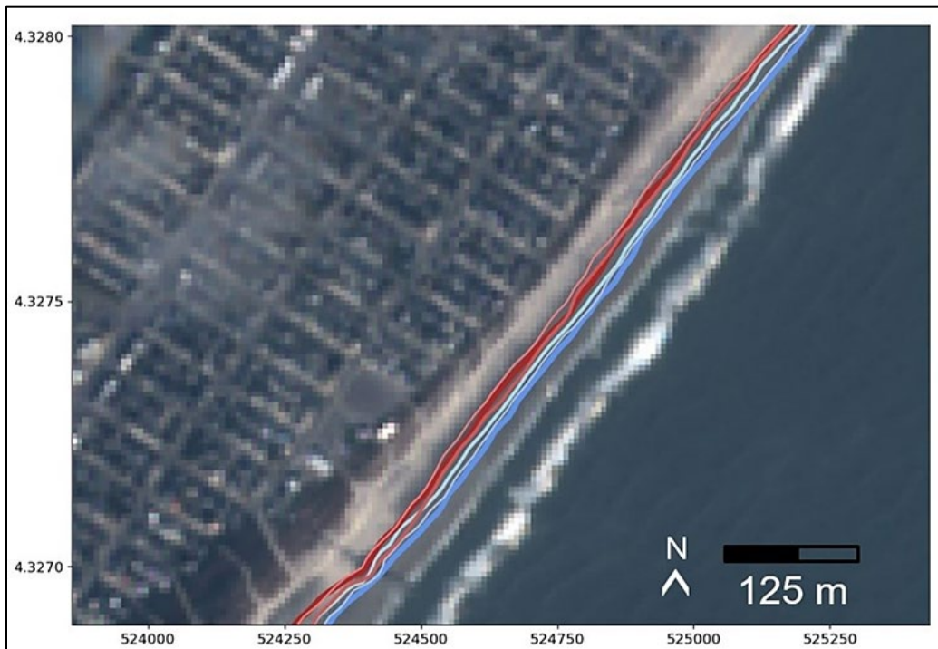
Figure 37. Satellite shorelines spanning from 24 August 2011 to 16 September 2011 with early dates in blue and post-Irene (25 August 2011 impact) shorelines in red . Note shoreline erosion on the order of approximately 50 m.
