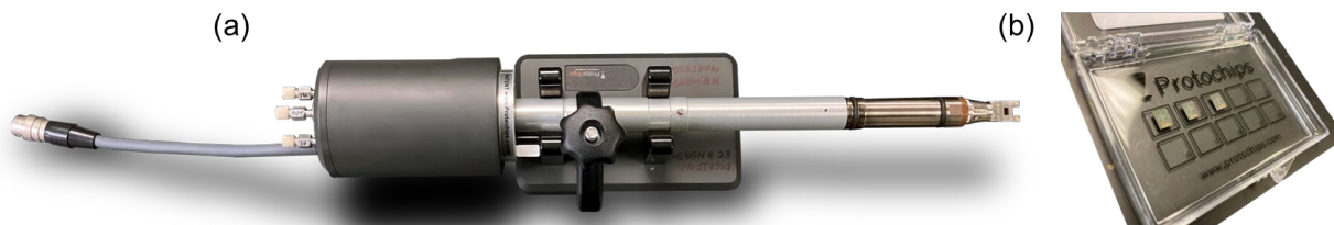
Figure 1: Photo of (a) the in-situ liquid cell holder with simultaneous heating and electrochemistry and (b) the MEMS chips compatible with the new holder design.
