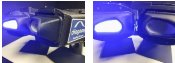
Figure 1. Novel ERG/pupillometer developed for this project. Note the two eye-cups allowing light to be applied to either eye independently. Cameras located in the eye-cups are used to record pupil size, and a nearby amplifier connects to ERG electrodes.
