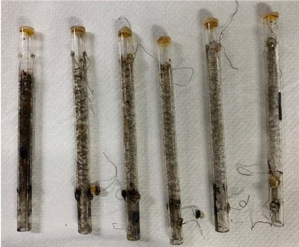
Fig. 3-2. Sample tubes after combustion of the gelled propellant mixture at pressures: from left to right, 4, 5, 6, 7, 8, and 9 MPa.
