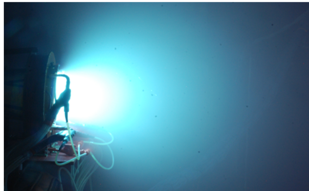
Figure 21: 10 s exposure image of the RMF thruster operating at the Large Vacuum Test Facility at the University of Michigan.
