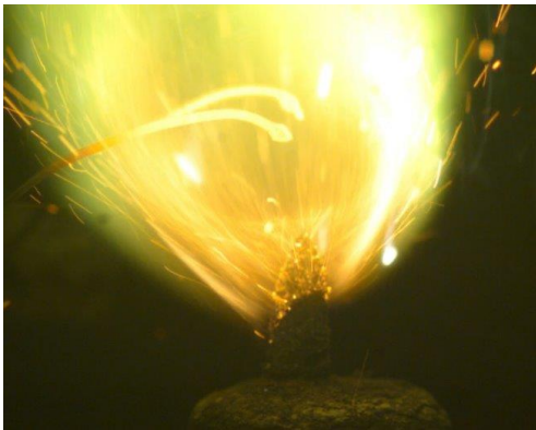
Figure 4. Still image of atmospheric combustion of HTPB/AP/MgB 2 (20/70/10 wt%).
