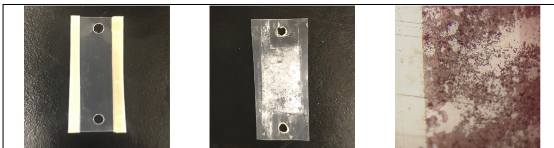
Fig 2. (Left) An unmineralized sample is shown with PEEK tapes sealing the edges. (Middle) A mineralized sample with lateral unmineralized regions. (Right) A zoomed-in image of a mineralized sample with calcium mineral deposits stained red.
