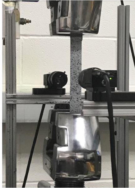
Figure 4. Digital image correlation and uniaxial tension test performed on AS4 carbon fiber specimen.
