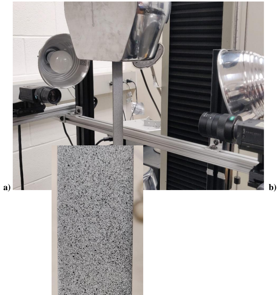
Figure 15. a) DIC camera setup with light sources b) speckle pattern
