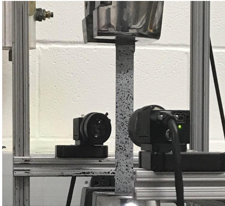
Fig 5. Tensile test on AS4 carbon fiber test coupon. Speckle pattern is applied to both sides of coupon. DIC cameras are placed on both ends of the coupon.
