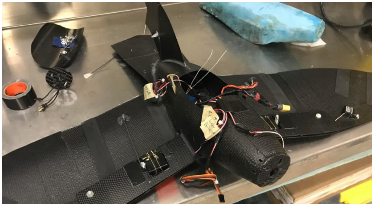
The sweep mechanism and tendon actuator mechanisms are illustrated in Fig. 5. Both mechanisms are to be actuated by servos positioned in the fuselage and attached via Kevlar strings. The strings will be wound around a nylon rod attached to the motors and supported by fixed bearings.
