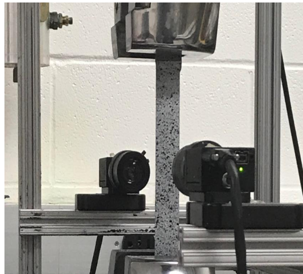
Figure 23: Tensile test on AS4 carbon fiber test coupon. Speckle pattern is applied to both sides of coupon. DIC cameras are placed on both ends of the coupon to average out through-thickness deflection.
