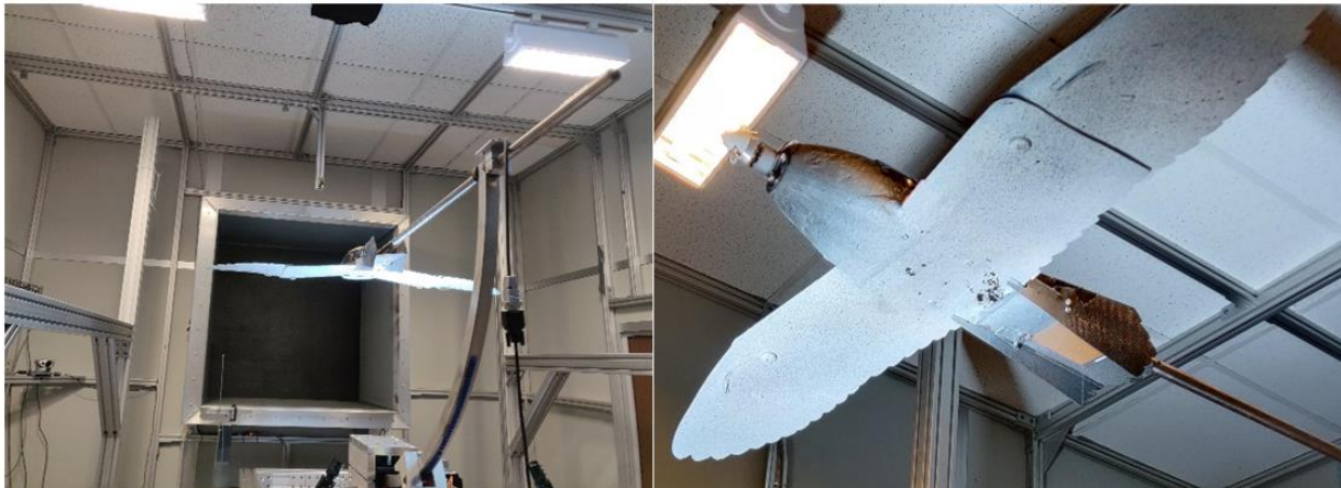
Figure 13. Wind tunnel setup with vehicle on mount (right) and Speckled pattern on wing of the test vehicle (left)
