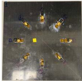
Ultra-strength CFRP - 305 mm × 305 mm × 3 mm
