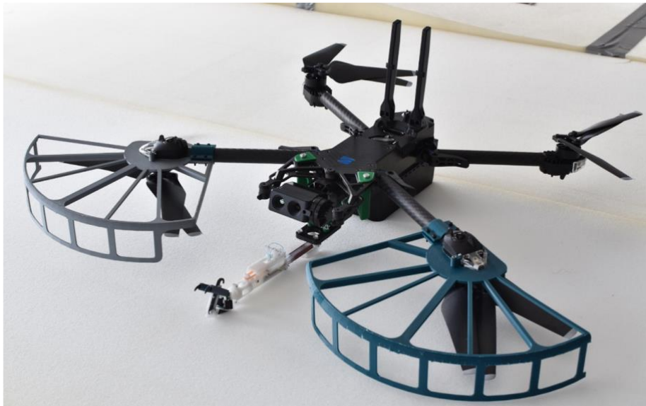
Figure S1 The integrated Skydio X2 vehicle with the Stanford gripper and other necessary modifications. 7
