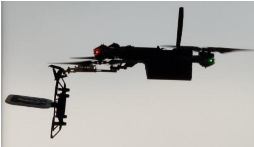
Figure S3 The Skydio X2 flying with a captured target drone. This demonstrates the capabilities of the X2 to adapt to the aerial grasping scenario.
