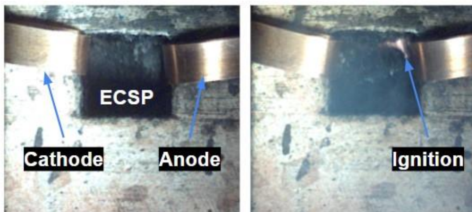
Fig. S2.9 ECSP with MWCNTs at initial state (left) and at ignition (right)
