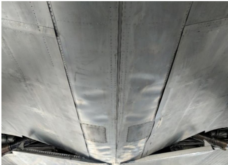
Figure 1: Permanently deformed panels on SR-71 at Museum of Flight in Seattle, WA.
