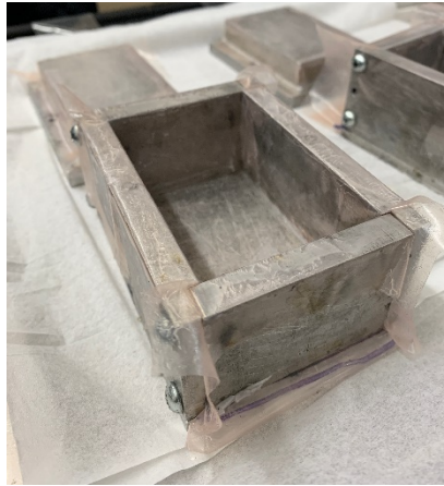
Figure 2.2: Single cavity aluminum mold for fabricating 3" X 2" X 1" PBS bricks.
