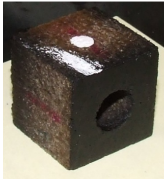
Figure 3.4: Neat PBS 8001 sample spray painted with layer of flat enamel black paint to ensure an emissivity of approximately 0.95.
