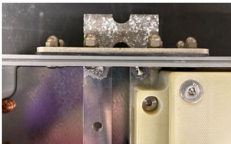
Figure 11. DCB sample mounted within the enclosure after 18 days of MDACT exposure.
