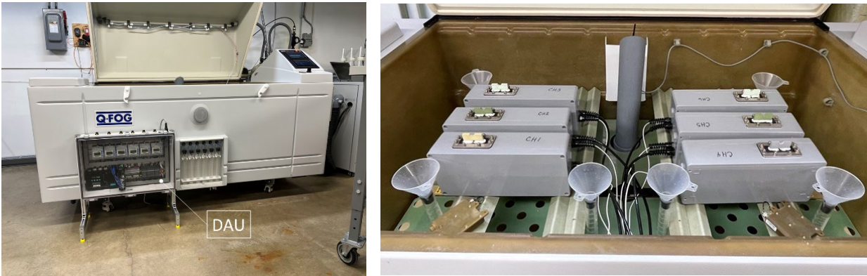
Figure 10. DAU and cyclic corrosion test chamber (left) and SLEAC load frames within chamber (left).
