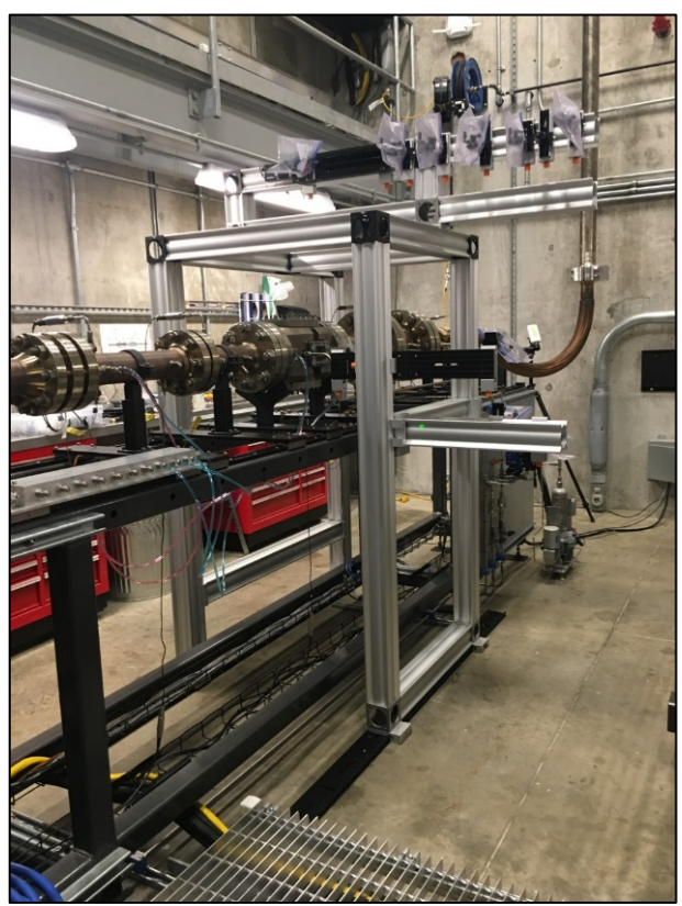
Figure 20: Photograph of the VIPER Test Stand with ACE assembly which will be used for the high pressure plasma-assisted burner.
