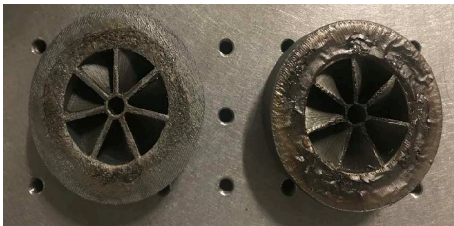
Figure 15: Evolution of swirler damage from exposure to the burner flame.
