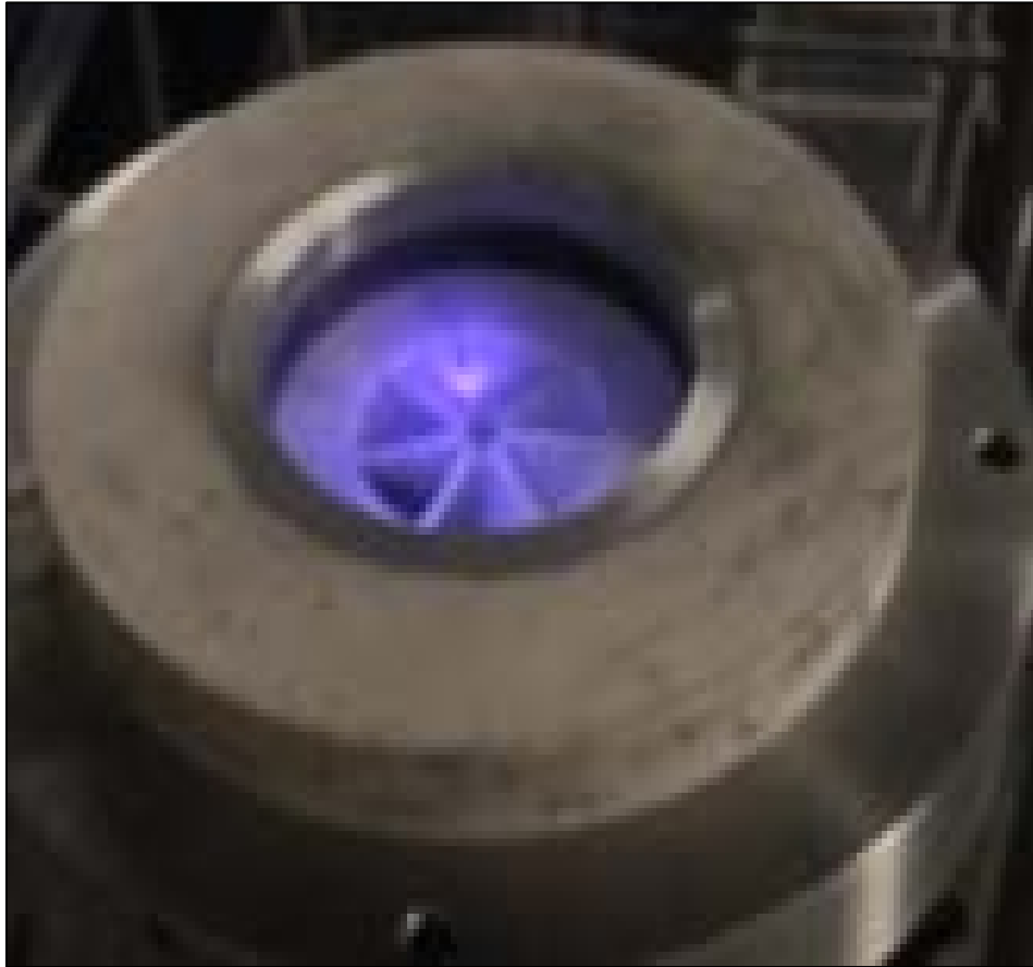
Figure 47: Diffuse plasma regime for an air flowrate of 300 SLPM.
