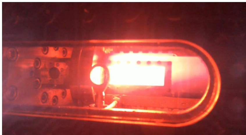
Figure 27 Overheated high-pressure swirl-stabilized combustor at 20 bar
