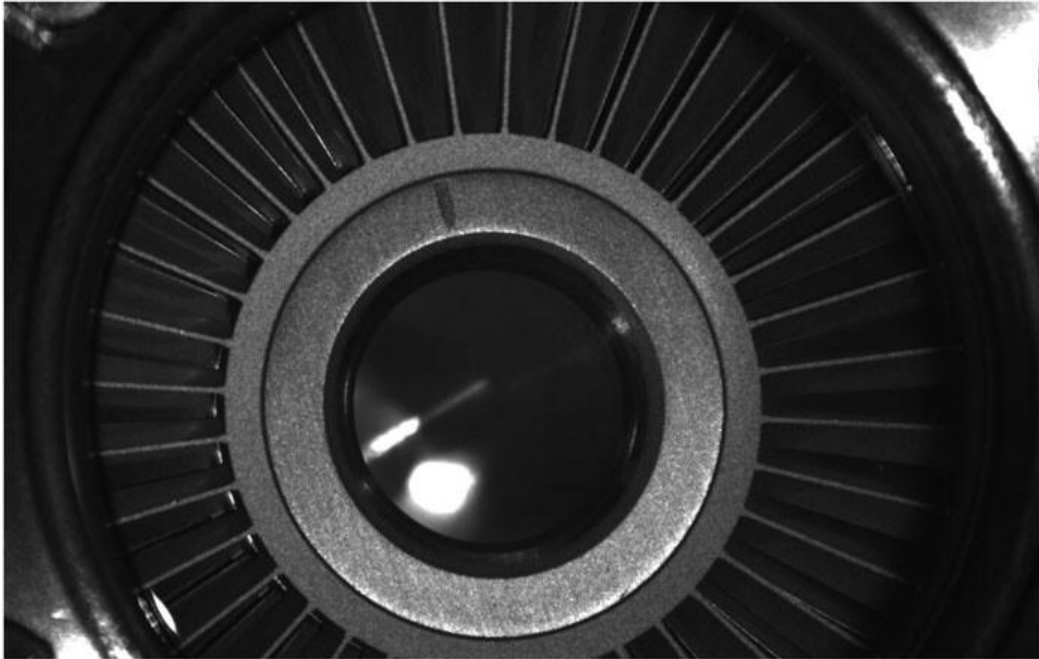
Fig. 2. One frame of a turbomolecular pump rotor stage operating with a rotational frequency of 56,000 rpm (corresponding to a velocity of 300m/s near the pump wall) acquired at a distance of 2 m with a spatial resolution of about 100 \mu\text{m} . The full video is available here: https://doi.org/10.1063/5.0076899.2
