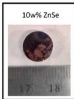
Figure 6. Composite sample disk of BG with 10% by weight of ZnSe particles coated with \sim 30 \text{ nm} of alumina.
