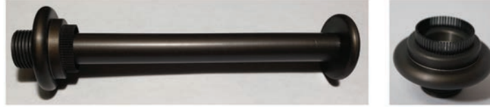
Figure 3. Photograph of the machined, anodized split cathode assembly (left) at UNM. Photograph showing the carbon nanotube emitters (right).
