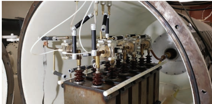
Figure 5. Photograph of the PI-110A accelerator used for MDO experiments showing solid state resistors in place.
