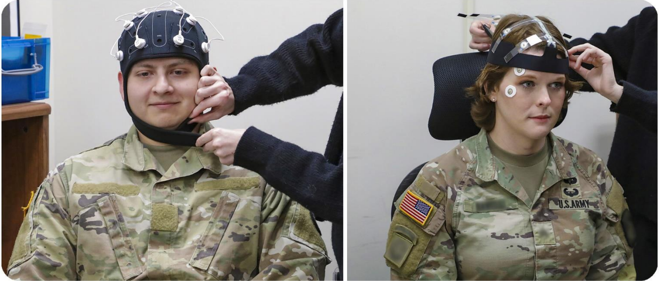
Figure 1. Depictions of EEG systems (left, StarStim; right, Advanced Brain Monitoring B-Alert) that include pre-defined electrode placeholders.
