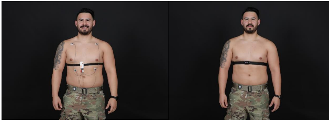
Figure 5. Examples of ECG recording setups (left, four-lead Shimmer device; right, band-only Polar H10).
