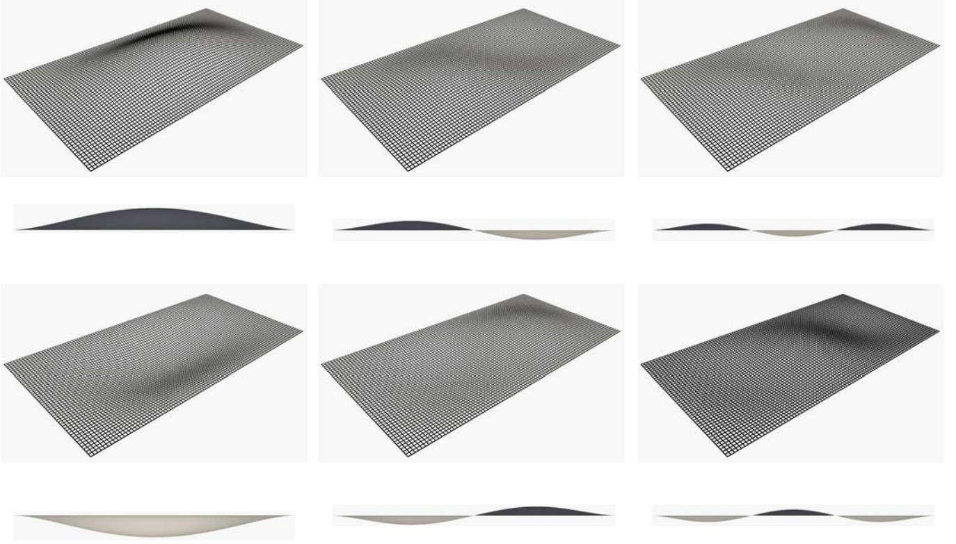
FIG. 19. Modes of deformation considered; rows: first +ve, second -ve; columns: modes 1, 2, and 3.
