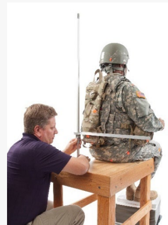
4. Modified anthropometer for height measurements
