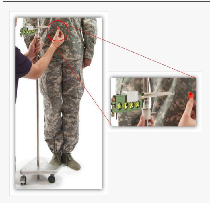
2. Modified anthropometer for measurement transfer
