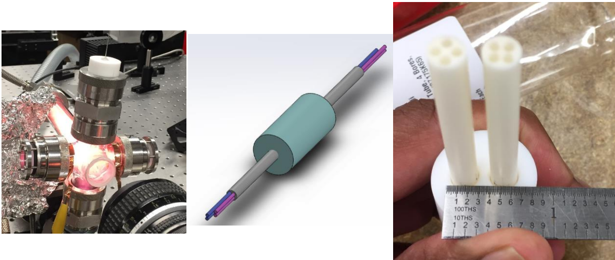
Figure 15: A Kanthal wire heater rated up to 1200 \text{ }^\circ\text{C} was used as a substrate. The metal substrate on the left was replaced with wire heater and thermocouples. 4-bore Ceramic tubes ( 1/4'' OD) were used to make the connections.
