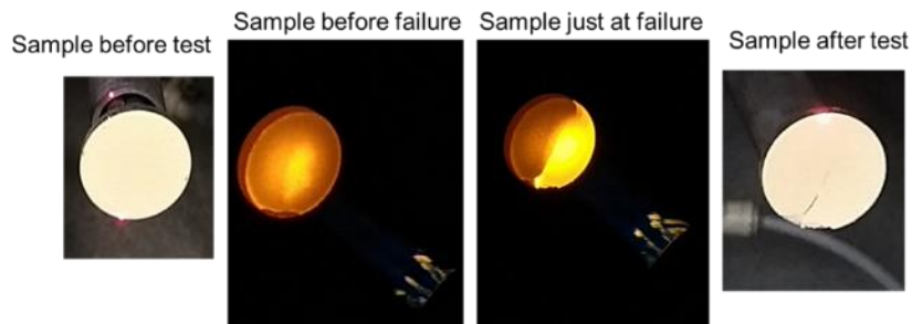
Figure 8. Images of a TBC sample at different stages of the Burner Rig test.
