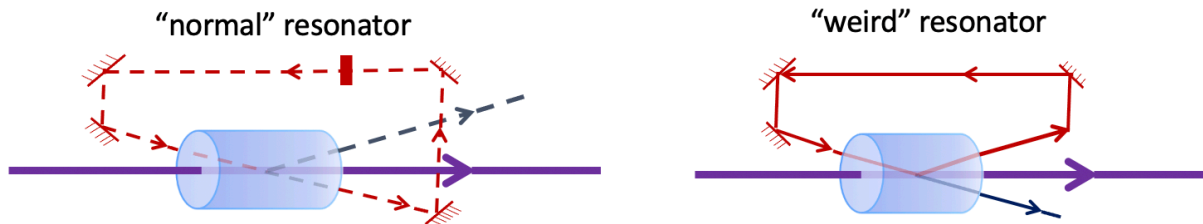
Figure 13. Ring resonators for optical parametric oscillators. (left) A normal singly-resonant OPO ring resonator with either the probe or conjugate frequency oscillating, selected by an etalon. (right) A phase-conjugate mirror resonator denoted “weird resonator” that circulates, alternately, the probe and its correlated conjugate frequencies. (In fact, both frequencies will fill the cavity simultaneously.)
