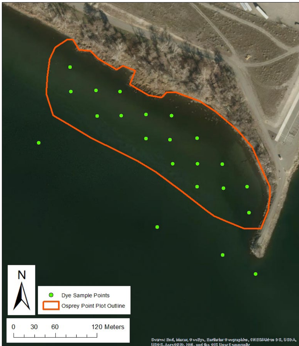
Figure 2. Outline of Osprey Point study plot with rhodamine water tracing (RWT) dye sampling points. Direction of river flow is Northwest to Southeast.
