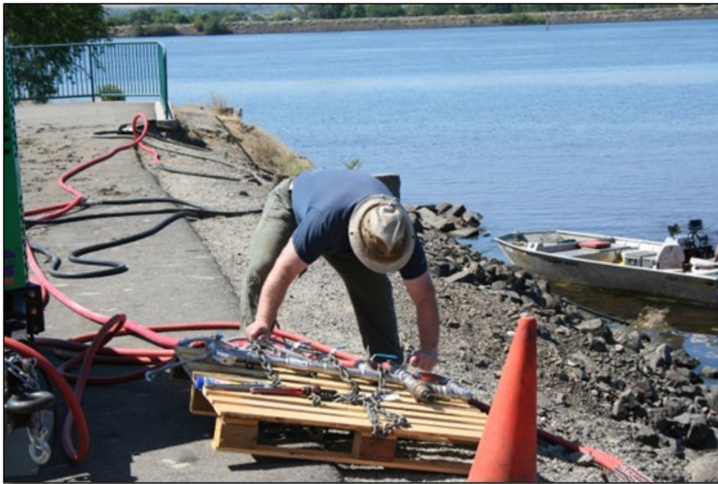
Figure 3. Six-valve manifold equipped with a pressure gauge and bleeder valve that provided constant air flow throughout each bubble curtain during the water exchange studies at Osprey Point in 2019.
