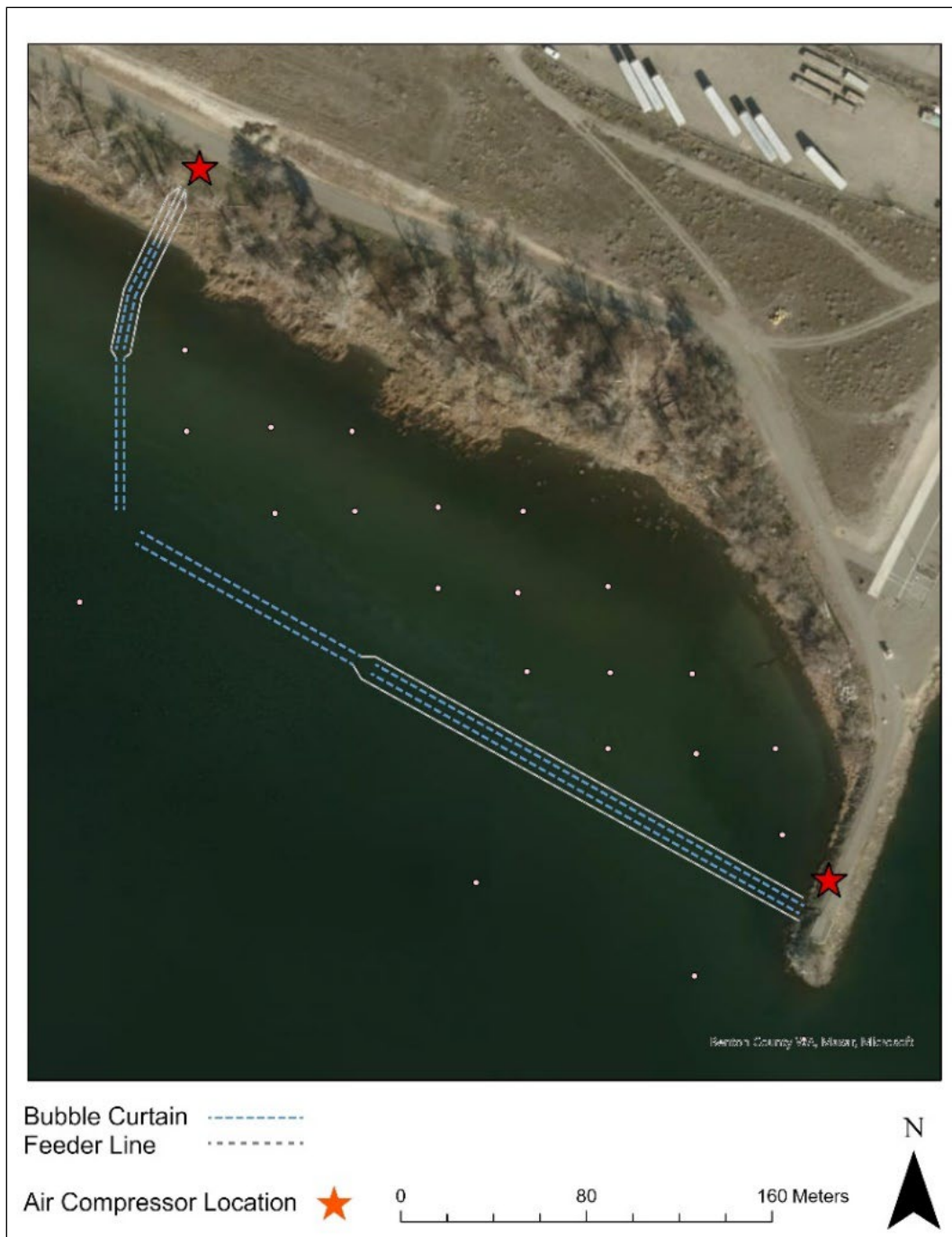
Figure 6. Arrangement of the double bubble curtain at the Osprey Point Study Plot on 26 July 2019. Direction of river flow is northwest to southeast.
