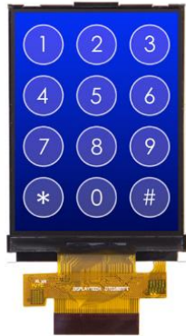
Figure 6-15: Example of Commercially Available Medium-Format, Direct-View Display Module
