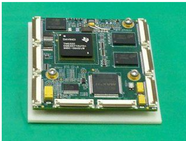
Figure 6-13: TI DaVinci SOC Integrated Into a Printed Circuit Board (PCB)
