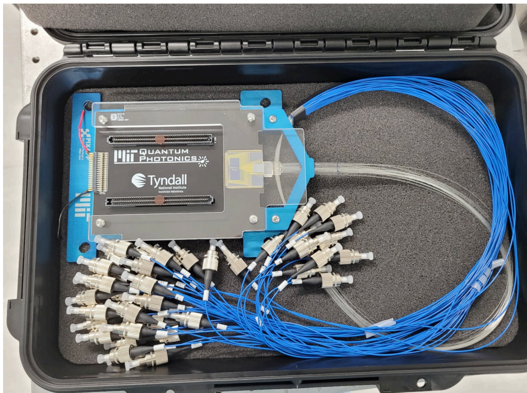
Figure 2. Photograph of the final packaged PMMI system. The 20x20 unitary photonic circuit is flip-chip bonded to a custom high-density silicon interposer, which is wirebonded to a high-resolution printed circuit board for easy interfacing
