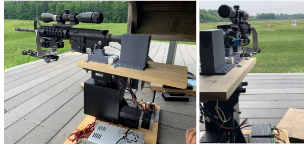
Fig. 6 ISW-FCT v1.0 mounted to XY position table
